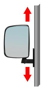
With the mirror in the correct position, use a marking device to mark the location of the mounting holes on the driver side front strut. Set the mirror in a safe location.
